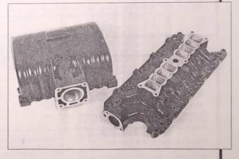
more power from modified stockers. In the February '93 Super Ford, as part of the Head, Intake and Cam article, we found one of JBA's hand-ported intakes came within 14.1 horsepower and 4.5 ft/lbs of a port-matched GT-40 on a 313.7 horsepower small-block. Furthermore, at 2500 rpm the JBA hand-port was 22.3 ft/lbs and 10.6 horsepower ahead of the GT-40, which says something about driveability and fuel mileage at street cruising rpm.
