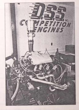
Valve timing was dictated by a Crane Cams emissions legal 2040 Compucam delivering .489-inch valve lift and 220 degrees of duration at .050-inch lift. Compatible Crane hydraulic roller lifters, hardened steel pushrods, 1.6 ratio roller rocker arms and part number 99838 valve springs installed to deliver 320 pounds of open pressure, along with Motorsport guide plates and Milodon rocker studs, completed the valvetrain.
