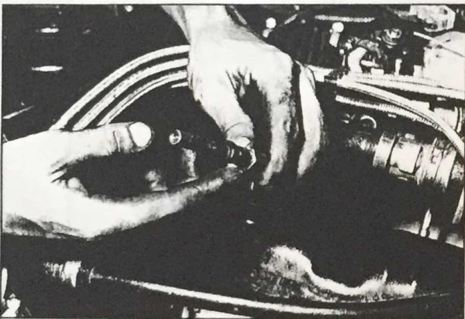
The injectors can be pulled now. There is a special removal tool for this procedure. In most cases it's wise to replace the O-rings around the injectors at this time.
