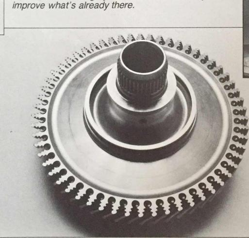
By varying pressure and abrasive grades, the Extrude Hone machine can polish metals as hard as steel gears.
