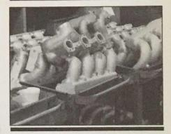
A vast array of Oldsmobile Quad 4 intake runners awaiting the porting process. Mixed in with the many Quad 4 units are various Porsche intakes and jet ski impeller housings. Each benefits greatly from the process.
