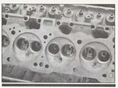
While the Extrude Hone process works well on cylinder heads it is probably not as cost effective as manual porting. Care must be taken to protect the valve guides from the abrasive media flow. All chamber work will still have to be performed in the normal manner.
