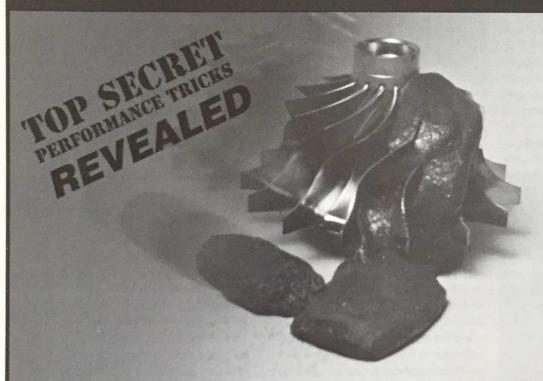
Used to lighten turbo wheels for faster response or port an intake system for maximum air flow, Extrude Hone Porting or Abrasive Flow Machining as it is also called, this 20-year old technology could be one of the major performance secrets of the nineties.
