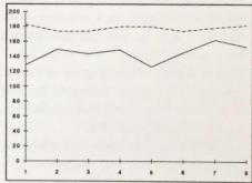
This chart shows not only the improvement of the overall air flow of the stock upper & lower combination (solid) to the Extrude Hone ported combination on a cylinder by cylinder basis. Note how much smoother the solid line is reflecting more even air flow to each cylinder.
