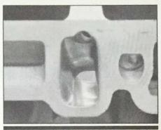
The port of the 5.0 Ford intake manifold after the Extrude Hone process. The media follows the path of the air flow. It removes material where it receives the most resistance (where the greatest flow obstructions occur).
