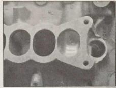
A 5.0 Ford lower intake after Extrude Hone porting. Note the overall conformity of the walls with no grooves or troughs left from the process. The media flow is in the same direction as the normal air flow. It does not leave radial grooves that often occur in hand porting.
